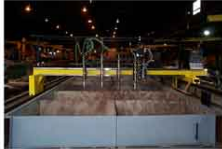
Burdox burning machine with a Burny 5, HT2000 Plasma punch marker and 4 oxy/fuel torches 10 ft. wide, 65 ft. long
