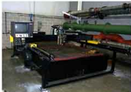
Heath burning machine with a Burny 10, punch marker, and HD3070 HyDef Plasma 6 ft. wide, 12 ft. long
