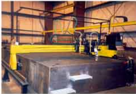
Airco burning machine with a Burny 5, Merlin 6000 Plasma, punch marker and 2 oxy/fuel torches 10 ft. wide, 40 ft. long
