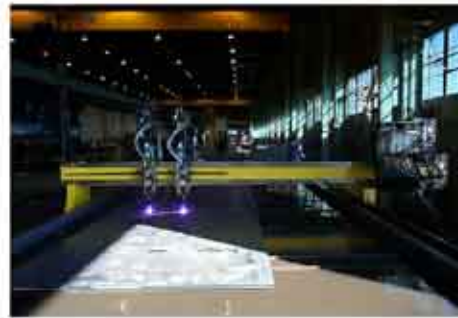
Burdox burning machine with a CMC Burny 3 controller 2 Hypertherm HT2000 Plasmas 10 ft. wide, 100 ft. long
