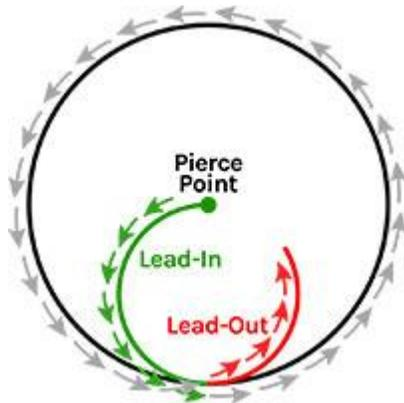
**Incorrect - Do Not Include A Circular Lead-Out on Holes**
